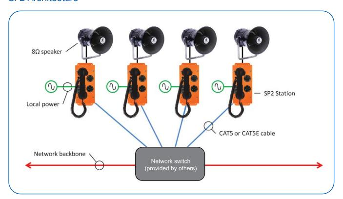
SP2 is simply wired to the nearest network switch using CAT5 or CAT5E Ethernet cable. Local power is supplied to each station either as a separate power cable or contained in a hybrid power/Ethernet cable. Simple screw terminals within the station make field wiring possible without the need for any special tools.
